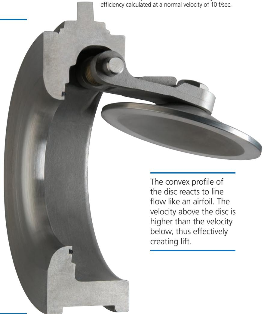
The convex profile of the disc reacts to line flow like an airfoil. The velocity above the disc is higher than the velocity below, thus effectively creating lift.
